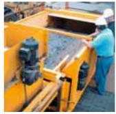
The combination of screening drum and Vibrosort generate a very good preliminary concentration of non-ferrous metal, by removing rubber and hard plastics in the Vibrosort. The fine particles of the inert fraction are screened out of the material flow and can be re-processed, if required.
