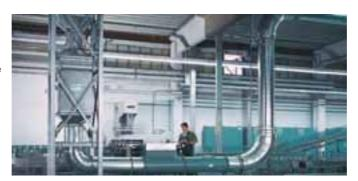
Great emphasis is placed on hygiene in the food-processing industry. For the drinks industry, for example, PET bottles are treated in our suction type PET bottle conveying plant. This makes it impossible for residual liquid or contaminated air to leak from the pneumatic conveyor system.
