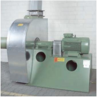
Fans which are continually exposed to extreme weather conditions or which operate in a humid medium can be provided with a hot-galvanised corrosion protection. We use fans made from rustproof or acid-resistant steel for chemically aggressive media.
